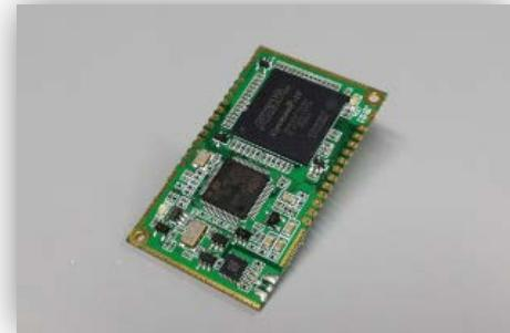
INNOS's Sync Detector WDM-C234V5 provides accurate TDD Timing directly generated from the RF signal.
